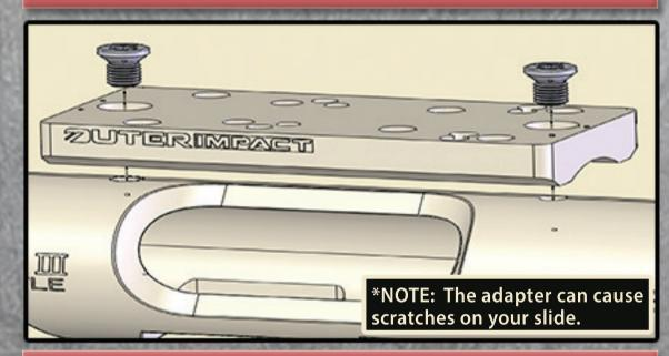
**Step 2:** Align M.R.A. as illustrated above. Fasten M.R.A. with torx screws. Torque to 25 in/lbs.
