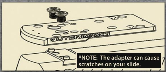
NOTE: THE ADAPTER BASE PLATE HAS AN INTENTIONAL CURVE. THIS CURVE WILL FLATTEN OUT WHEN MOUNTED TO THE FIREARM.
